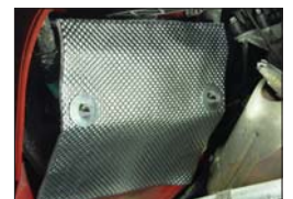
Protects electrical connections from engine and exhaust heat
