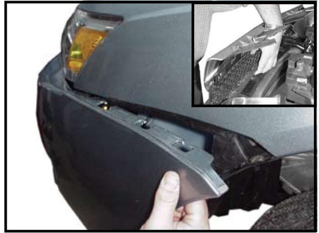
5. Pull fascia out by wheel well on each side and lift up behind grill and carefully slide fascia off.
