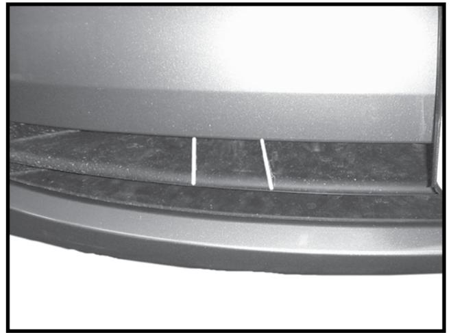
11. Mark where the pull ears will pass through fascia and cut out plastic bar in fascia as shown in picture.
