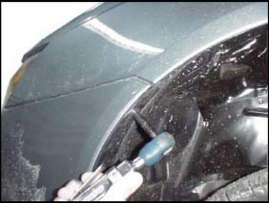
2. Remove one screw from each wheel well.
