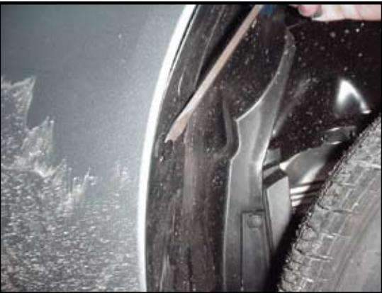
3. Remove two plastic push fasteners from wheel well to fascia on each side.
