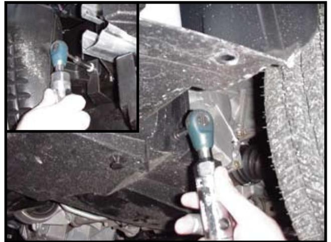
6. Remove plastic filler panels from each side. One screw and four plastic push fasteners on driver's side, and one screw and seven push fasteners on passenger's side and remove one bolt from air box.
