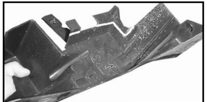
7. Cut passenger's side plastic filler piece as shown in picture.
