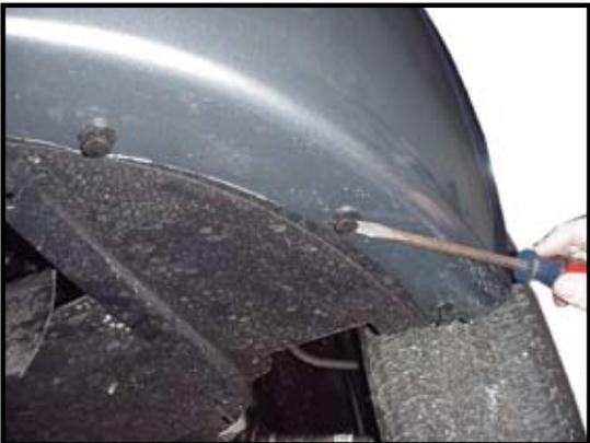
4. Remove three plastic push fasteners from bottom side of fascia to wheel well extension, on both sides.
