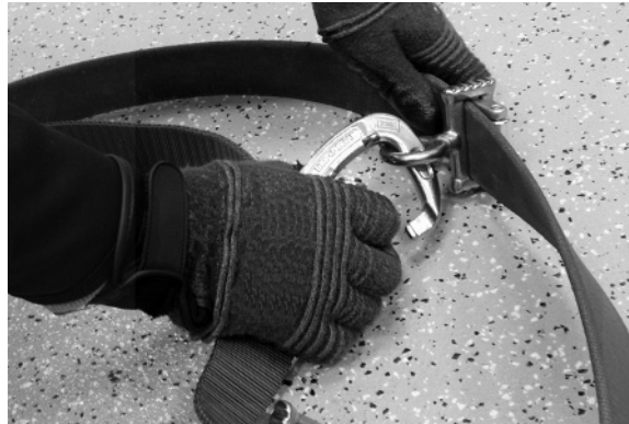
Figure 50 - Rope or Web Lanyard , Disconnect Captive Eye Carabiner from Cynch-Lok Roller Adjuster
