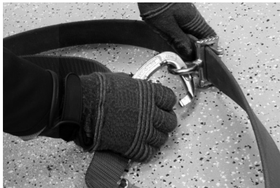
Figure 43 - Web or Rope Model, Connect Captive Eye Carabiner to Cynch-Lok Roller Adjuster
