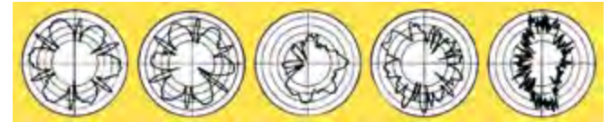
DAVIS ECHOMASTER #152 DAVIS EMERGENCY RADAR REFLECTOR #151 MOBRI RADAR REFLECTOR FIRDELL BLIPPER RADAR FLAG Strong peaks, narrow valleys, and 360° returns are desirable.
