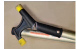
West Marine® snapped at 550 lbs. (249 kg).
