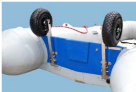
#1482 Wheel-a-Weigh Standard with 10" (26 cm) inflatable tires.
