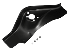
591053 (L) Repair panel 591054 (R) for inner wing
