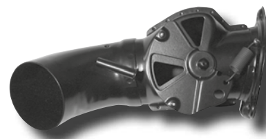
90.005 (1623200170) left (OE 911.211.013.01) Heat control box, long version (suitable for models with electrical heat control) Painted aluminized steel
