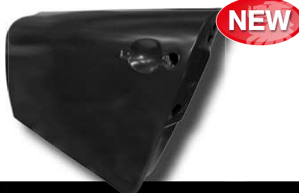
591041A (1680700470) left (OE 911.531.005.00) Door, complete 69-7/72 Painted steel
