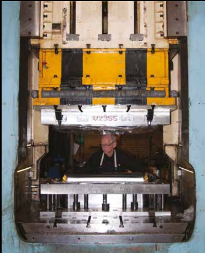
400 ton deep draw hydraulic pressing machine
