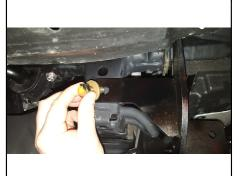
5. Insert 5/8" carriage bolts through the hitch mounting plates and tow loops. Secure hitch to tow loops by attaching supplied spacers and 5/8" flange nuts to carriage bolts.
