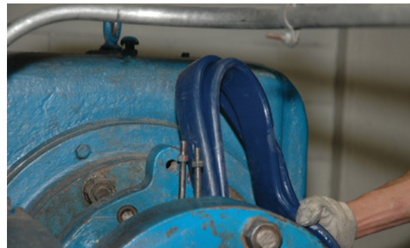
The outer silicone material is fed through the machine in the same fashion as the center core cover, eventually making it's way onto the wire and completing the forming process.
