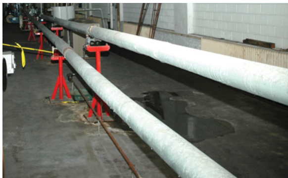
The wire travels 250 feet through these long tubes on the right in order to cure and cool the wire after manufacturing.
