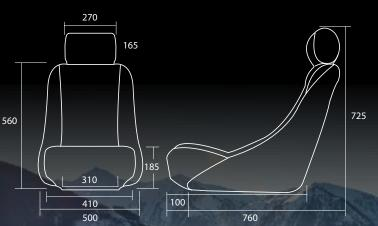
Each of the seats have been designed with a subtly tapering back to enable them to fit into smaller cockpits, but lower side supports mean that most drivers don't even realise that they are sitting in a narrower seat. These seats also feature a longer seat cushion - making them ideal for deeper cockpits.
