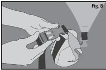
Included with your cover is a toss bag to help you attach the straps under your RV. Before you begin fill your toss bag with rocks or something of equal weight equivalent. Clip the toss bag to the buckle strap attached to the tension panel (Fig 8). Now toss the bag under your RV to the buckle on the opposite side (Fig 9). Unclip the strap from the bag and buckle the bag to the next strap. Repeat with the remaining straps.
