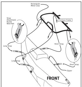
Now attach the two inside and two outside webbing straps on the pontoon to the pontoon frame. Thread the straps as follows:
