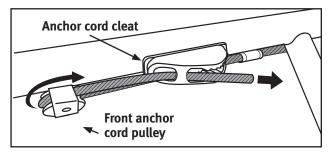
while anchoring, simply pull the cord into the jaws of the cleat. Pull up and away from the cleat jaws to release.
