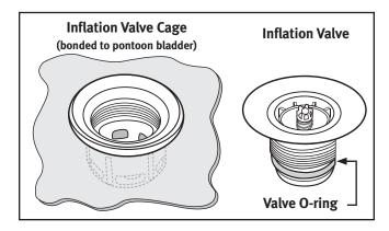
The inflation valve consists of a two-part assembly. There
