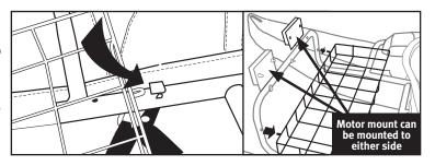
Attach the rear corners with two clevis pins. These secure the wire cargo deck and the rear platform frame to the pontoon frames. Be sure to insert each pin through the cargo deck, the rear platform frame and through the pontoon frames. Lock both clevis pins.
