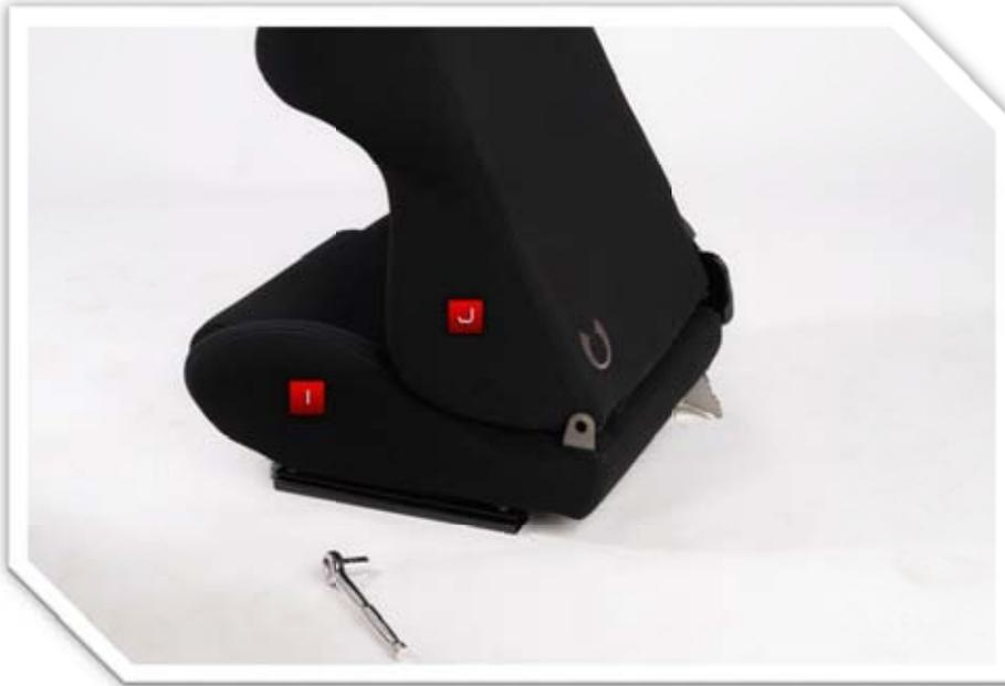
5. Align the single bolt hole on (J) with the hole on the metal tab on (I).
