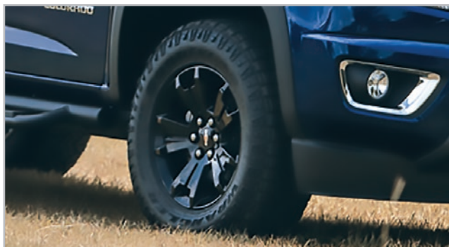
17-Inch Black Aluminum Wheel shown with Goodyear Wrangler DuraTrac Off-Road Tire D E
