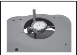
FIRST CHECK BELLHOUSING FOR BORE CONCENTRICITY. INSTALL MAGNETIC BASE TO FLYWHEEL OR PRESSURE PLATE, THEN INSTALL THE INDICATOR TO MEASURE THE BELLHOUSING BORE (SHOWN ABOVE). RO-TATE THE CRANKSHAFT AND MARK DOWN THE INDICATOR READINGS (MARKING THE BELLHOUSING WORKS WELL). THE MAXI-MUM OUT OF CONCENTRICITY IS .005".
