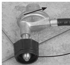
(B) Nipple has to be centered into the LP tank valve
