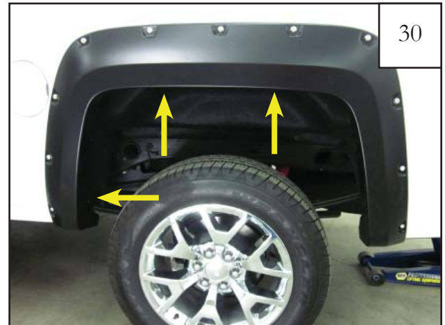
30 Hold rear flare up to wheel well to confirm fit. While holding flare on vehicle, install supplied screws (SW1-0056) into the 2 upper and 1 lower factory hole locations. Do not fully tighten at this time.
