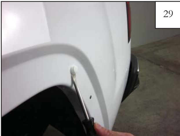
29 Use a pry tool to remove any remaining factory fasteners that may have stayed on the vehicle during the removal process.
