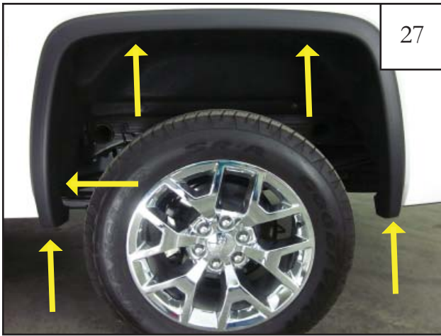
27 Remove fasteners from factory wheel arch molding using a T-15 Torx Bit for upper and lower wheel well fasteners and a 10mm deep socket and wrench for the lower 2 locations.
