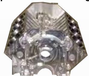
Front Timing Cover Lightening
