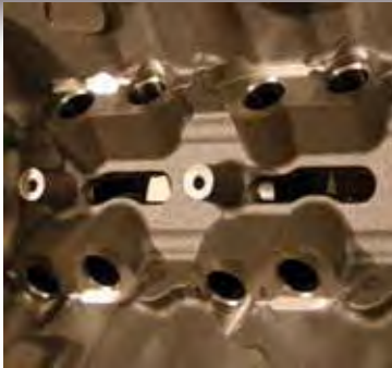
LIFTER BORES AVAILABLE: .842 OR .903 BORE DIAMETER
