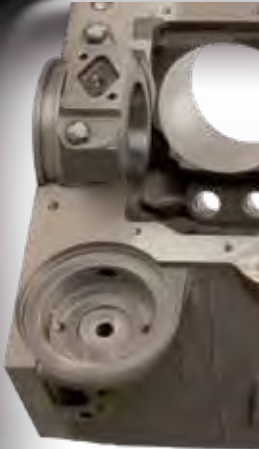
OIL FILTER MOUNTING BOSS IS DESIGNED FOR BOLT-ON OIL FILTER ADAPTER
