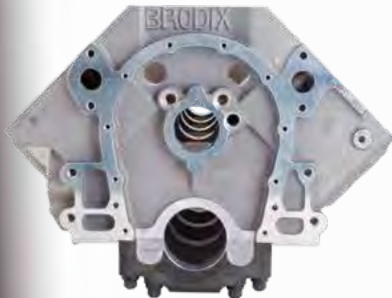
BILLET MAIN CAPS INSTALLED WITH SPLAYED BOLT PATTERN
