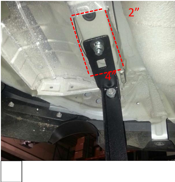
Fig 1 STEP2: Starting from the Passenger Side, remove the muffler from the chassis.
