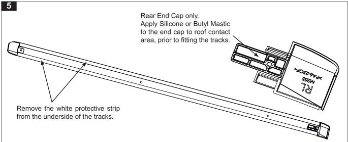
Place the tracks into the roof gutters, cutout to the rear, pointed edge to the outside of the vehicle. Front screws only. Assemble the spring washer and flat washer onto the M6 x 20 security screw, insert into the front track hole and screw into the roof nutserts, leave loose. Engage the middle and rear screws into the remaining nutserts progressivelly tighten all three screws.
