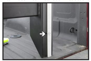
1. Attach the plastic rails using the appropriate hardware to the hitch base and space according to the trucks bed ribs, leave loose.
