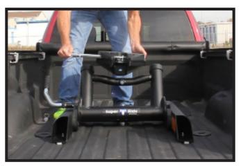
5. Set the hitch head on top of the shock towers.
