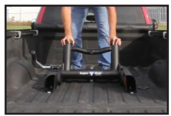
4. Move the shock towers towards the cab of the truck and manually reengage the locking handle.
