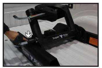
The handle is now locked into the grove on the side of the tubing.
