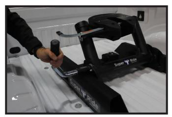
Release locking handle by pulling the handle towards the rear of the truck bed.
