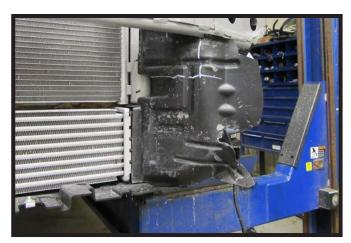
5. Using a reciprocating saw, trim the marked areas on the bumper plastic shielding.
