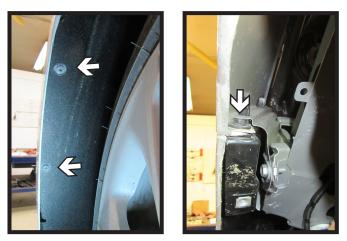
2. Using a T15 Torx, remove the two screws from the edge of the wheel well in front of the tire. Next, pull the cover back. Using a 7MM socket, remove the one (1) bolt from under the cover. Do this for both sides of the vehicle.
