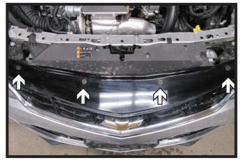
1. Using a 7MM socket, remove the four (4) bolts from the top of the fascia cover.
