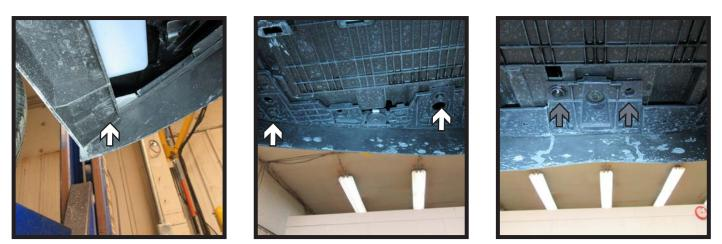
3. Using a 7MM socket, remove the six (6) bolts (white) from the underside of the vehicle. There are three (3) on each side of the car. Remove the two (2) push pin (gray) from the center of the underside.
