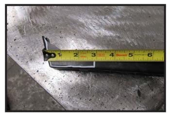
12. Before reattaching the front brace. Mark brace 3" from bottom corner then down and across as indicated. Do this for both sides of the brace. Then using a recipricating saw trim marked area to allow the brace to sit further back on the baseplate when reattached.
