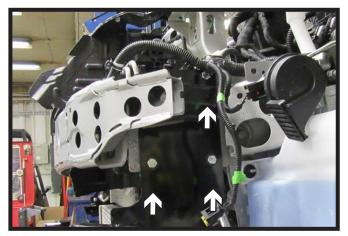
Using a 3/8" drill bit, drill out the remaining three (3) holes and insert the provided 3/8" hardware. Do this for both sides of the vehicle.
