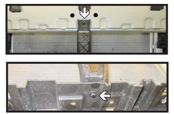
7. Using a 7MM socket, remove the two (2) bolts from the brace on the front of the fascia. One (1) from the top and one (1) from the bottom fo the brace.
