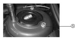
■ Install the new spring strut upward and screw on the top nuts (5).
