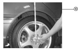
■ Lower the vehicle approx. 400mm (axle centre – lower edge of the fender) from the lifting platform (1).
