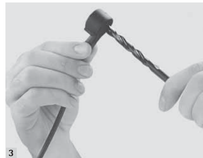
3 Drill 8 mm hole on the pulse timer (turn drill by hand).
