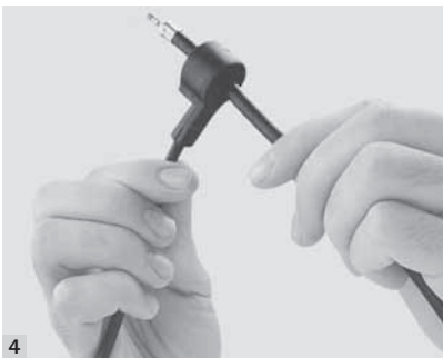
4 The ignition cable with the M3 connection can now be pushed through the pulse timer.
