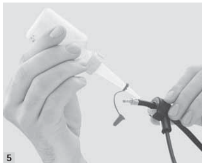
5 Now lubricate the ignition cable with installation oil.
