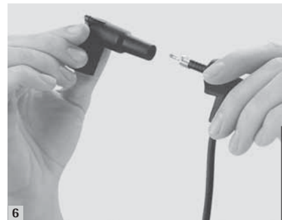
6 Finally, screw on the ignition distributor connector of the CopperCable.
