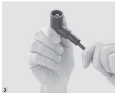
2 Unscrew the ignition distributor plug on the new CopperCable (spray with installation oil).
