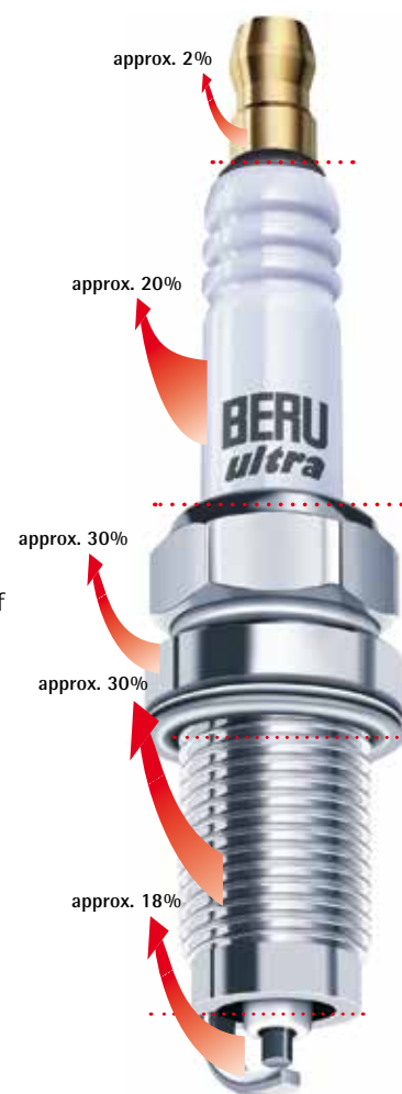
Heat conduction path of a spark plug
