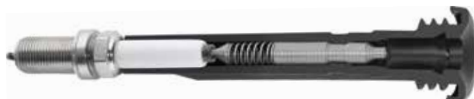
Greater flashover resistance in spite of higher ignition voltage: thanks to the longer insulator neck, the greater overlap, the recessed pressure spring and the new contact technology.
