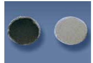
Carbon deposits in the filter paper three minutes after the cold start. With post-heating (on the right), carbon deposits are approx. 40% less than without post-heating.
