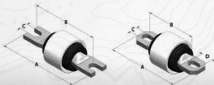
"BP" BAR PIN MOUNTING DIMENSIONS EB1 WITH BUSHING AND BAR PIN
