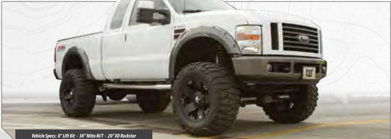
Vehicle Specs: 8" Lift Kit - 38" Nitto M/T - 20" XD Rockstar
