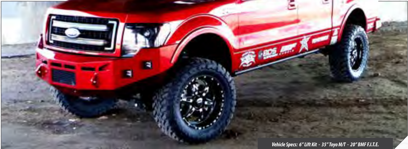
Vehicle Specs: 6" Lift Kit - 35" Toyo M/T - 20" BMF F.I.T.E.
