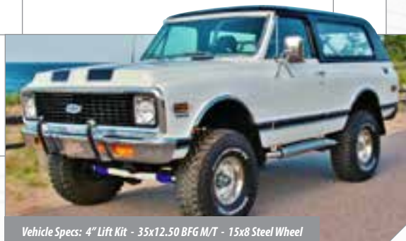
Vehicle Specs: 4" Lift Kit - 35x12.50 BFG M/T - 15x8 Steel Wheel
