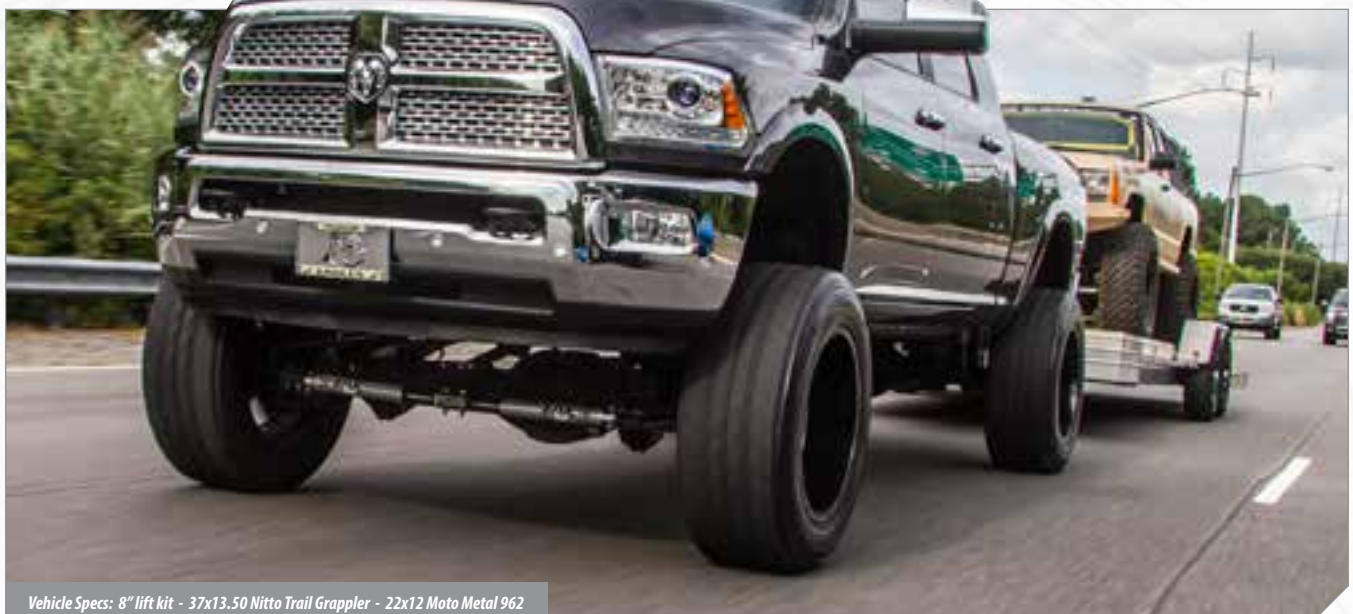
Vehicle Specs: 8" lift kit - 37x13.50 Nitto Trail Grappler - 22x12 Moto Metal 962
