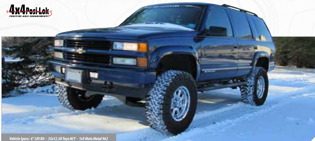
Vehicle Specs: 6" Lift Kit - 35x12.50 Toyo M/T - 1x9 Moto Metal 962
