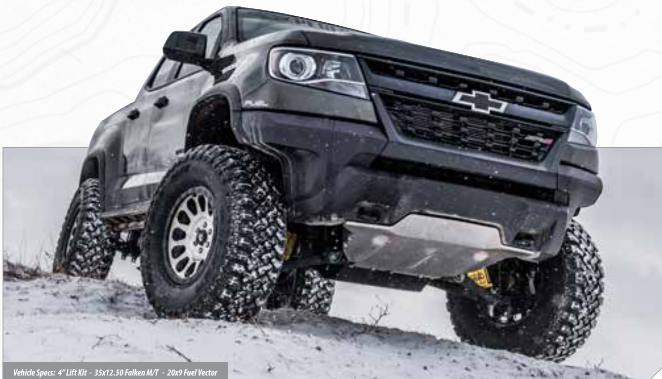
Vehicle Specs: 4" Lift Kit - 35x12.50 Falken M/T - 20x9 Fuel Vector
