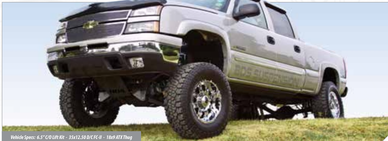
Vehicle Specs: 6.5" C/O Lift Kit - 35x12.50 D/C/FC-II - 18x9 ATX Thug
