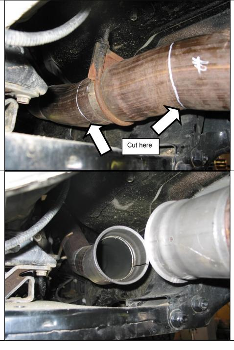
Cut out the marked pipe section using a reciprocating saw or cutting disk. Remove any burrs left on the edge of the pipe using a file or similar tool, then slide the pipe adapters onto the two cut ends of the pipe. Install the brake valve between the two exhaust pipe adapters using the two supplied V-band clamps. Ensure the exhaust pipe adapters are in line with the brake valve to prevent possible leakage.
