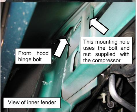
**Note** On 2013-2017 trucks there is an air intake tube inside the fender. This tube ends before the BD compressor bracket, but it may still be easier to install the compressor assembly with this tube removed.
