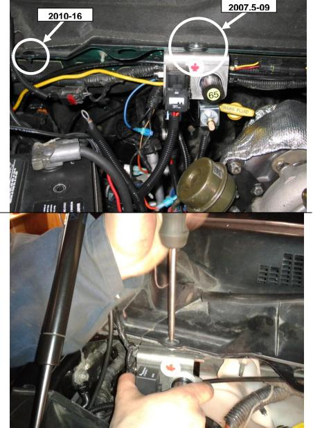
2010-2017 Vehicles Remove the plastic trim clip or wiring harness clip on the top of the firewall near the coolant bottle. This hole will be used to install the regulator assembly.
