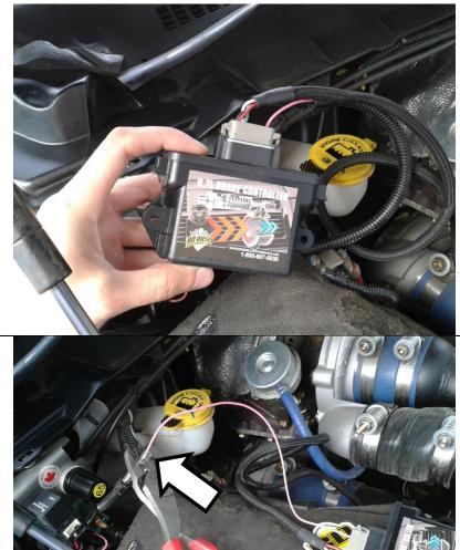
Connect the pink trigger wire from the module harness to the air regulator assembly's pink wire using the pre-installed butt connector.
