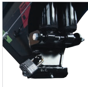
Lockable BULLDOG® coupler for added security
