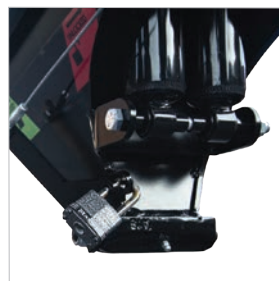
Lockable BULLDOG® coupler for added security
