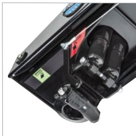
Automatically locks when coupling
