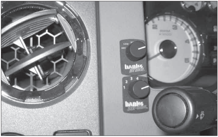
Figure 21 Finished installation of the Six-Gun/Banks Brake Switch
