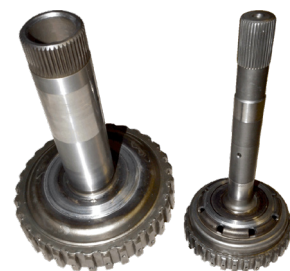
Overdrive/Forward Clutch Hub Dodge Ram 68RFE
