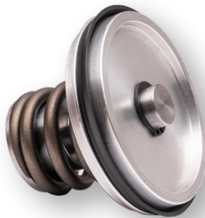
47/48 Billet Reverse Servo Piston Kit (aka L/R Accumulator) P/N: 3140142104
