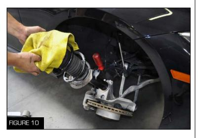
11. Be sure to cover the top of the strut with a towel and then push down on the strut and brake assembly to get the strut out (Figure 10)
