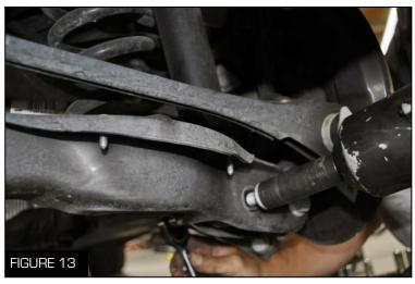
3. Using the 18 mm socket and wrench, unbolt the inner bolt connect the shock to the suspension arm (Figure 13)
