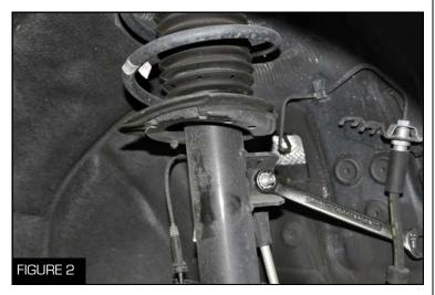
3. Unbolt the sway bar end link using a 14 mm socket/wrench (Torx T30 bit may be needed) (Figure 2)
