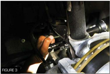
1. Properly jack up the vehicle on flat, level 4. Unbolt the lower bolt that holds the strut in wrenches (Figure 3)
