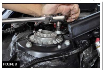
10. Using the 14 mm socket wrench, unbolt the 12. Be sure to use a spring compressor when strut bar and using the 16 mm socket wrench removing the OEM spring and when putting the unbolt the 3 bolts holding the strut in place, and ARK lowering springs on (Figure 11) then lower the strut down (Figure 9)
