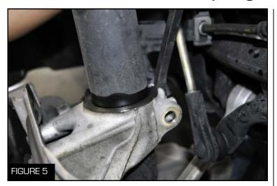
6. Use the pry bar to push the clamp apart and let the lubricant soak in (Figure 5)
