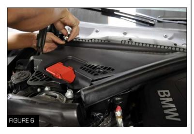
7. Using the 10 mm, remove the battery cover (do the same thing for driver side) (Figure 6)
