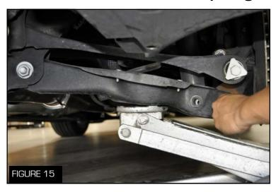
5. While supporting the suspension arm with the jack, remove the outer bolt and then slowly lower the jack (Figure 15)
