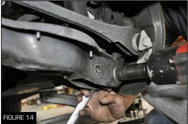
2. Unbolt the lower tray using the 10 mm socket | 4. Using the 21 mm socket | and wrench unbolt the outer bolt on the suspension arm (Figure 14)
