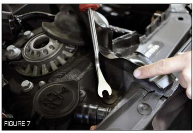
8. Using the clip remover, take out the clips that hold the rubber cover down over the strut/strut bar (Figure 7)
