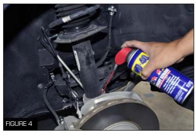
5. Spray a lubricant on the strut/clamp to make removal easier (Figure 4)
