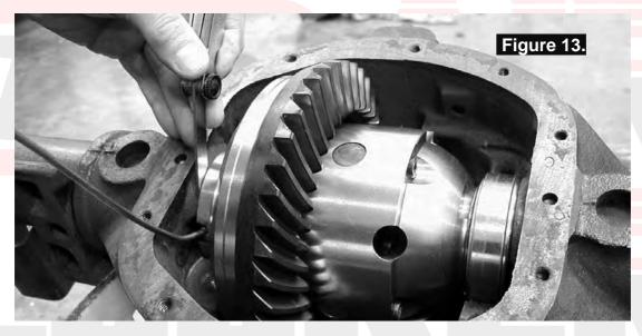
Consult your vehicle manufacturer's service manual to determine the carrier bearing pre-load amount specified for your vehicle.
