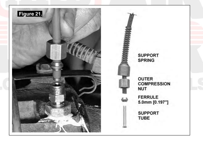
Insert the support tube all the way into the end of the air line.
