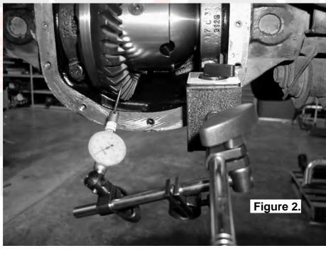
While supporting the pinion gear by holding the drive shaft flange, rotate the differential in both directions while observing the maximum variation in depth from the indicator (i.e., the highest value minus the lowest value). This value is referred to as the ring and pinion backlash.
