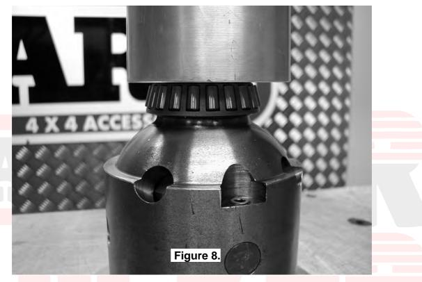
] Invert the *Air Locker* and press the other tapered roller bearing cone onto the opposite bearing journal of the differential carrier until the bearing seats firmly against the bearing journal shoulder.
