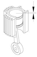
Deck height should measure between 0.50mm and 0.70mm [0.020 and 0.028"]
