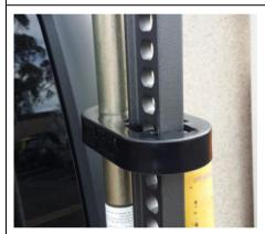
Install handle keeper (Part No. ARB203HKB/ARB203HKR) to Hi-Lift jack to eliminate handle rattle.
