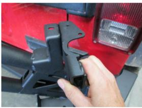
21. Install Hi-Lift bracket. Use Bolts M8 x 20, M8 Spring Washers, M8 Flat Washers and M8 Flange Nuts. Do not tighten fully.
