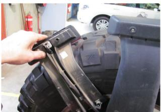
7. Remove O.E. wheel holder from vehicle and retain all components. Remove and un-plug stop light housing.
