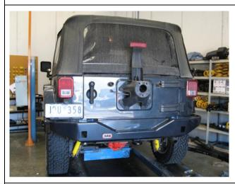
6. Fit (Re-fit) Rear bar to vehicle as per fitting instructions (Part No. 3789186) Steps 7 – 14.
