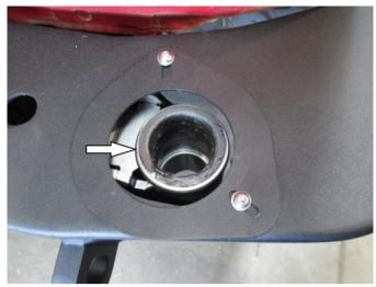
9. Lightly grease pivot bush bore and top face.
