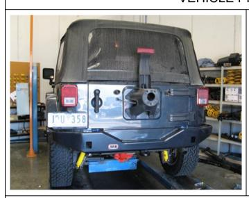
1. If vehicle is already fitted with ARB Rear Bar (Part No. 5650360) remove in reverse order of fitting instructions (Part No.3789186 - stopping at step number 5). If ARB Rear Bar is not yet fitted carry out steps 1 – 5 from Fitting Instructions (Part No. 3789186).
