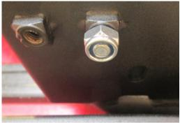
Install M10 Nyloc Nut from underside of Hi-lift Jack Support Plate onto the M10 knob. (The Nyloc Nut is to reduce the chances of the M10 knob falling out if left loose). It is important the Nyloc Nut is fully engaged on the thread of the M10 Knob.
