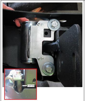
5. Install Pivot Bushing onto Rear Bar using M12 x 90 Bolts, ½" Spring Washers, M12 Flat Washers, Crush tube (on lower bolt).
