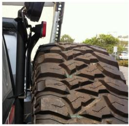
28. ALL MODELS. Place wheel mount into arm and secure using two M12 x 35mm bolts, M12 spring washers and M12 flat washers into cage nut plate (slide in through rear of carrier). Leave finger tight. Place wheel on mount ensuring it is inflated as per vehicle tyre placard and tighten all components so inner edge of tyre is sitting on Lightpost Tyre support face.
