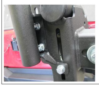
Do not tighten fully. It will be necessary to fit Spare Wheel Mount and adjust height of Light Post to suit before tightening bolts once desired height is achieved.
