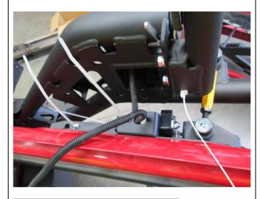
32. Run wiring along desired route and use supplied cable ties to fasten to carrier arm and light post.
