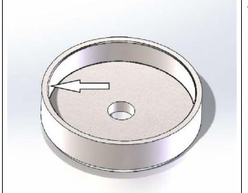
12. Lightly grease inside bore of Shaft Sealing Cap.
