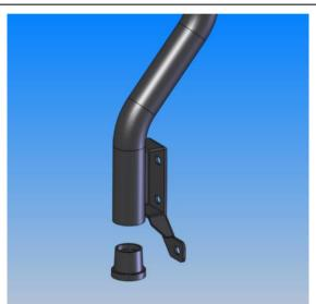
24. Install light post rubber plug on tube end.
