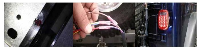
Connect one side of the resistor to the plate The other end of the resistor will get Inside the taillight assembly.
