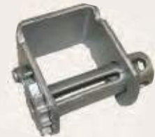
43565-127-XZ Storable Bottom Mount X-Treme Zinc Finish C Track Slider Lighter 7mm heat treated frame Weight: 8.2 lbs./3.7 kg. WLL: 6,000 lbs./2,730 kg.
