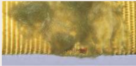
Excessive abrasive wear
