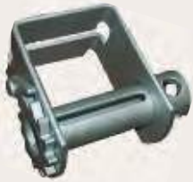
49207-127-XZ Storable Double L Track Slider X-Treme Zinc Finish Lighter 7mm heat treated frame Weight: 6.8 lbs./3.1 kg. WLL: 5,500 lbs./2,500 kg.
