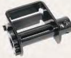
49207-137 Standard Double L Track Slider Lighter 7mm heat treated frame Weight: 6.5 lbs./2.95 kg. WLL: 5,500 lbs./2,500 kg.
