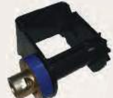
43565-157-RW Slider Ratcheting Lighter 7mm heat treated frame Weight: 9.1 lbs./4.1 kg. WLL: 6,000 lbs./2,730 kg.
