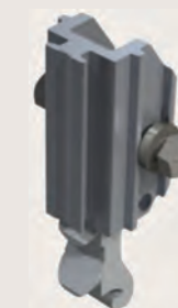
50187-31 Lift-A-Deck II Low Profile Foot Assembly. Machined guide shoe allows for inspection of both locking lugs while beam remains installed in the track. Features a coil spring for optimum service life. Weight: 0.6 lbs./27 kg.
