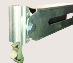
50187-30 Lift-A-Deck II Low Profile Foot and Tube Assembly. Machined guide shoe allows for inspection of the locking elements while foot is installed in track. Features a coil spring for optimum service life. Weight: 3.1 lbs./1.41 kg.
