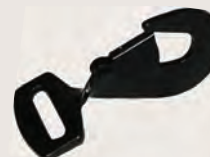
40758-11 2-inch Snap Hook w/ Satin Black Finish. Twisted Version WLL: 3,333 lbs./1,515 kg. Weight: .59 lb./27 kg.
