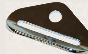
49968-10 2", 45 degree Heat treated, Chrome Plated Finish. WLL: 1,000 lbs./450 kg. Weight: .10 lbs./05 kg.
