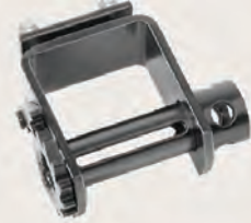
43564-127 Web Storable Portable w/ 2SS Weight: 11.1 lbs./5.0 kg. WLL: 5,500 lbs./2,500 kg.
