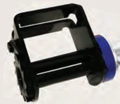
49207-137-RW Standard Ratchet Winch Double L Track Slider Lighter 7mm heat treated frame Weight: 8.0 lbs./3.6 kg. WLL: 5,500 lbs./2,500 kg.
