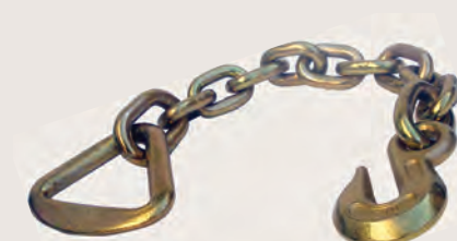
43366-14 Chain Anchor with Delta Ring for 3" & 4" Strap Assemblies. 3/8", G43 Chain and 3/8" G70 Grab Hook, gold zinc plated. WLL: 5,400 lbs./2,450 kg. Weight: 3.4 lbs./1.54 kg.
