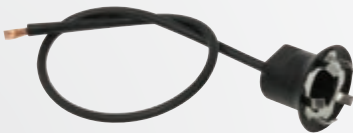
500127 Single Contact Socket Self Grounding Uses a standard 1895 bulb. Design to fit into a 5/8" hole.
