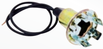
500157 Metal Tail Lamp Single Contact Socket Uses standard 1156 bulb. Design to fit into a 1-1/8" hole.
