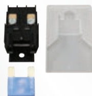
500449 "MAXI" Fuse Holder with 60 AMP MAXI Fuse Nylon plastic holder with white opaque cover. Comes complete with 60 amp fuse and has provisions for either a single screw mount or a clip. Large 10-28 screw connector will accept ring terminal or spade terminal.
