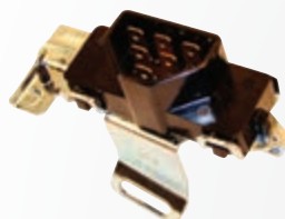
01993624 64-66 Chevelle, 64-66 GTO 63-66 Fullsize Turn Switch Assembly, all with tilt wheel
