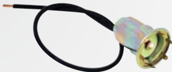
500125 Single Contact Socket Self Grounding Uses a standard 1895 bulb. Design to fit into a 3/4" hole.
