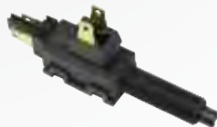
500145 Mutli-Purpose Brake/Cruise Switch Button type for use under dash. Has two blades for brake connection and two for use with cruise control, transmission lockup power or any device that requires a circuit interrupt when brake is applied. 1/2" mounting hole. ..... 12.00 ea
