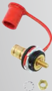
500010 Battery Jumper Stud Positive, with insulated cover. 3/8"-16 threaded brass stud mount. 13/16" dia x 1-1/8" long. Requires 1-9/32" hole. ..... 17.00 ea
