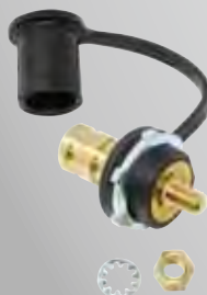
500011 Battery Jumper Stud Negative, with insulated cover. 3/8"-16 threaded brass stud mount. 13/16" dia x 1-1/8" long. Requires 1-9/32" hole. ..... 17.00 ea
