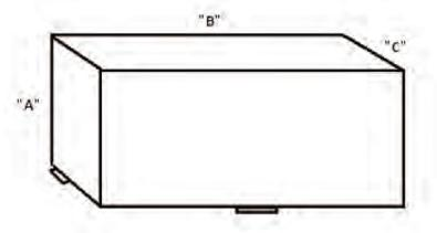
AUX51 is 55" across bottom - Sides of tank taper in at bottom
