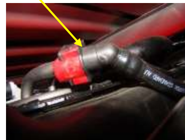
Fuel Tank Suction Tube
