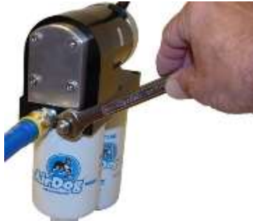
Loosen the Jam Nut Re-Torque After Adjusting
