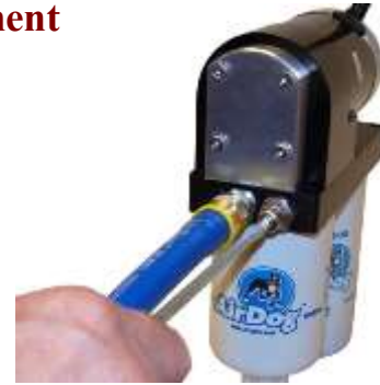
Use a Screwdriver to Adjust the Pressure Regulator
