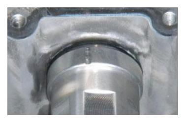
9. Rotate rear ring so the machine notch is straight up. Angled side is towards rear of engine block and o-ring. Tighten tube by hand until it has tension on front and on the rear o-ring.
