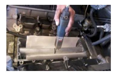
2. Cut cooling tube and remove rear part by hand.
