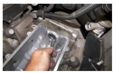
6. Remove rear o-ring in back of engine block.
