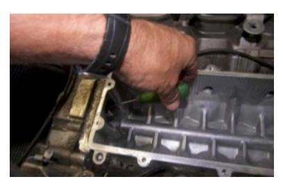
5. Remove old seal w/pick tool. Seal groove must be completely clean, use a small wire brush to remove ALL debris from old seal, inspect with mirror.
