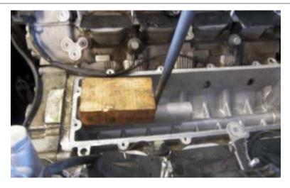
4. Pull tube out with lever bar.
