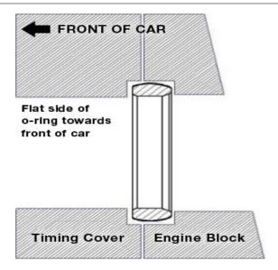
7. Install engine block front seal. Flat end of the seal should be facing towards the front of the car when installed in engine block.
