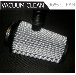
You can vacuum your Pro Dry S filter and return it to 96% of its original airflow. Remove the filter from the intake kit and vacuum away the dirt using a shop vacuum or regular house vacuum. Reinstall the filter in your vehicle. Do not apply oil to the filter.
