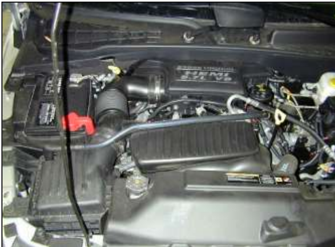
Factory air box system installed
