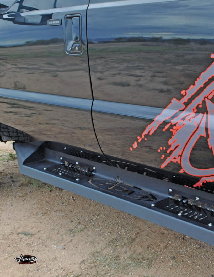
The Addictive Desert Designs Stealth Side Steps are as innovative as the name suggests. These steps feature step plates that can be color matched for a truly custom look and raised dimple holes to help with footing in the harshest of conditions. Combine the step plates with the multi-purpose accent lighting and you have steps that will not only help you locate your truck but also help locate the step itself for easy access in the dark or night.
