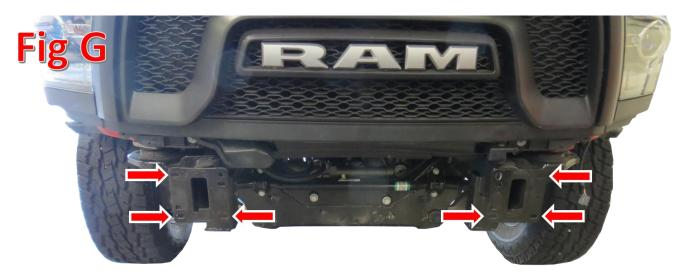
b. Secure the bumper to the truck using the supplied 1/2" Bolts (x6), 1/2" Washers (x12), and 1/2" Lock Nuts (x6). Leave these bolts finger tight for now. If you are keeping your tow hooks on the truck, use the bottom two bumper mounting bolts on each side to hold the hooks in place. (Fig H)
