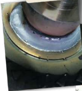
We spray weld for 6 to 8 times the strength. We also use Pulse Welding for greater control of the converters durability.
